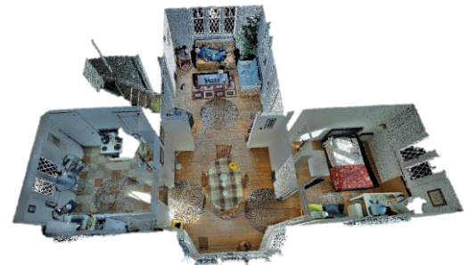
Figure 1 - A 3D image of the Crime Scene house at the University of Toronto Mississauga created using a laser scanner. Source: Eugene Lisio, AI2-3D. ( http://ai2-3d.com/ )
